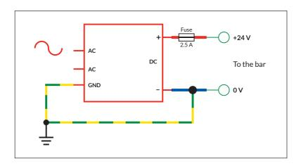
The 24 V supply connection (Pin 1, brown wire) must be fitted with a 2.5 A fuse. It is recommended that a type 'T' or 'gG' fuse is used.
