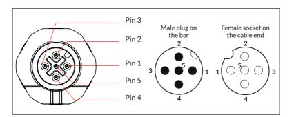
The pin assignment and typical wire colours are given in the table below. The table refers to cables supplied by Fraser. Other cables can have different colour schemes.
