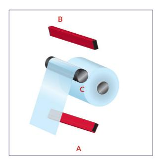
If there is a lay-on or contact roller (C), the best position for the XIFOS 33 is on the side where the film leaves the lay-on roller - in this case the underside (A) - because it can neutralise the charge as soon as it is created. If this is not practical, then position the bar on the top side. (B)
