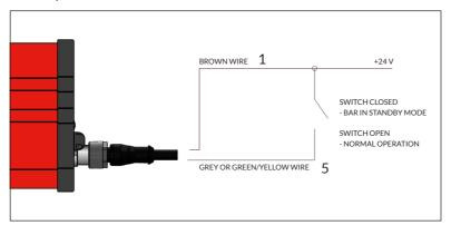
In Standby mode the internal HV supplies of the bar are disabled, the status LEDs flash red, and the OK output is inactive (open circuit) to indicate that ionisation is disabled. The DISABLE signal has a weak internal pull-down resistor, thus if the DISABLE signal is left disconnected the bar will operate normally.
