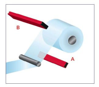
On a centre winder the XIFOS 33 may be positioned above or below the reel. It is a good idea for the ionisation to be directed mainly at the reel, but also catching the single sheet, as shown at (A). Position (B) is also acceptable.
