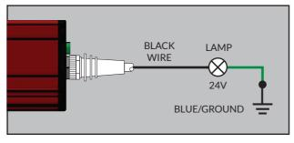
External indicator can be connected to BLACK wire to show status. This is useful for bars mounted in inaccessible areas.
