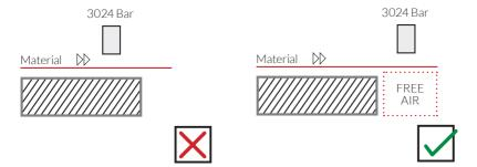
iii. The emitter pins should face the material to be neutralised and be within the following operating distance:
