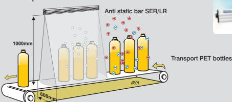
There are 3 different frequencies available to synchronise the system with the speed of the production machines. The high voltage unit is mounted in the anti static bar, enabling it to utilise 100% of its effect directly at the problem area without any loss of effect that a high voltage cable running alongside the machine would suffer. The voltage in the cable connecting the central unit and the high voltage unit of the system is only 24V.
