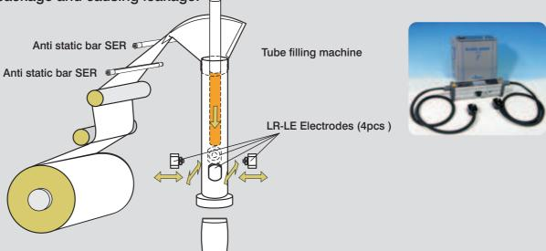
The **LR system** can even be used as a complete Static charge system, with the central unit supplying either a charging bar with integrated charging generator or a charging unit which can connect separate charging electrodes.
