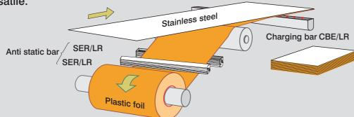
The process of coating sheets of stainless steel with a protective plastic foil to avoid scratches when piling or rolling the sheets requires 2 outputs from the central unit to discharge the plastic foil with an anti static bar on each side. This station ensures that the plastic foil always has the same charge (neutral) when it approaches the charging station. This ensures a repeated, optimal charge against the steel sheet at every cycle.
