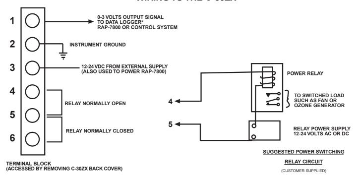
The C-30ZX internal relay is a low power device. It will handle up to 30 volts AC or DC at up to 1 amp so it will switch low voltage alarms directly. For switching power loads an intermediate relay and power supply should be used such as shown above.
